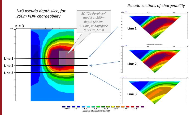
3D IP Forward model for a chargeable buried body shows responses over the "target" but also on lines near but offset from the "target". Interpretation of a single survey line has some degree of inherent ambiguity.
